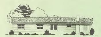
Best use of wall space for arranging furniture, cabinets, and household equipment requires three window sill heights. Varying sill heights detract from the exterior appearance unless they are skillfully blended with the walls of the house. Bold horizontal lines, created by raking the mortar from the horizontal joints and by flushing the mortar in the vertical joints, maintain integrity of line to give a pleasing horizontal emphasis at 8-inch height modules.
